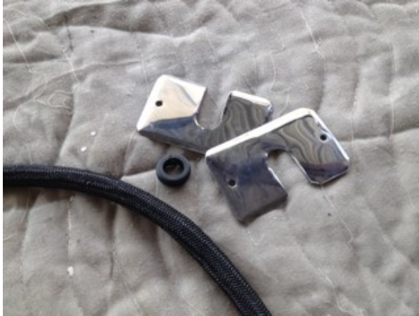
Figure 21 Firewall Penetration Parts
