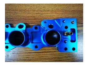
Drill and tap two M6 holes to attached expansion tank bracket.
