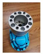
Step 3: Screw in 6pc M8x35mm bolts to the lugs you just inserted in the gearbox flange. Make sure it is fully tight and lugs have been pulled through. Use blue loctite and torque to 20 ft-lbs.
