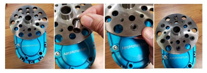
When using prop extensions, you must use the Rotax 4" or SAE-1 pattern. Both of these require you to install drive lugs in the gearbox prop flange. Figure 1 shows these being installed in the Rotax 4" pattern. If needed these can be drawn in place using a bolt and a stack of washers with an ID larger than the drive lug. Our props and extensions for the AM13 and AM15 use the Rotax 4" pattern.
